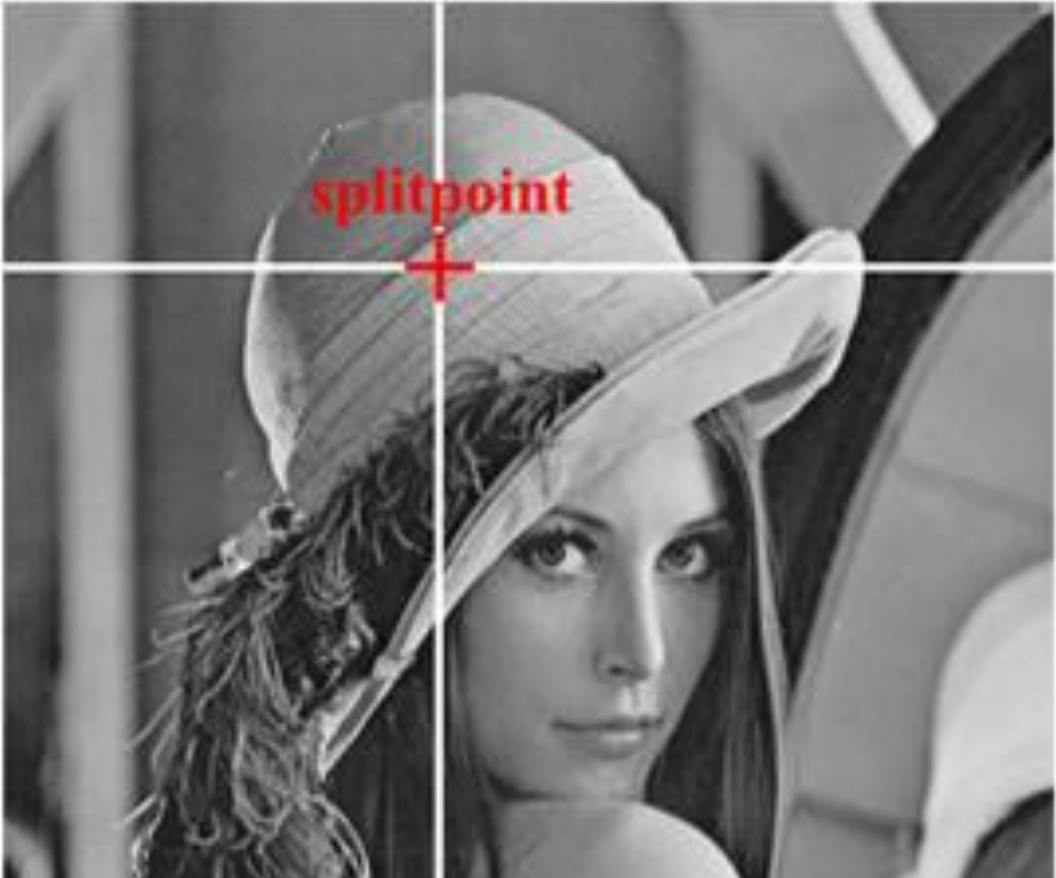
Figure 3. Sub-images resulting from splitting the input image at the optimal split point
